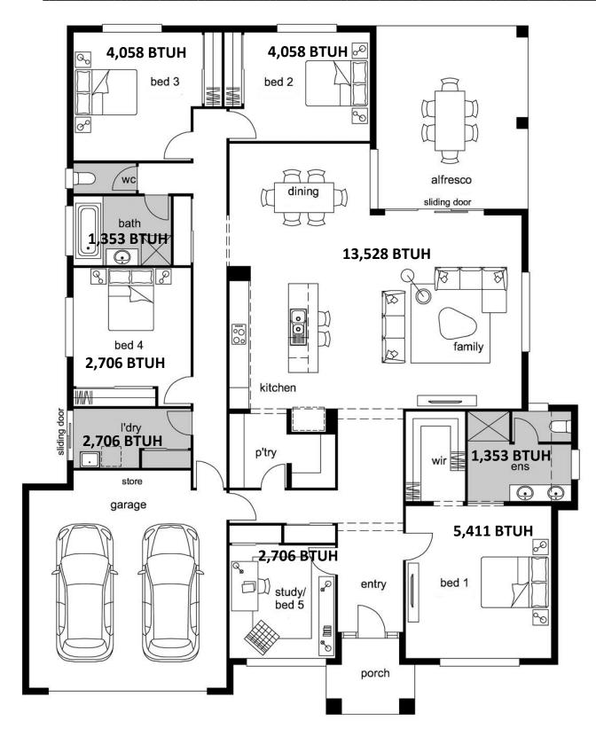
The Room-By-Room Cooling Load calculation has been completed for the home used in HW#5 and the room loads are shown on the plan on the previous page.
