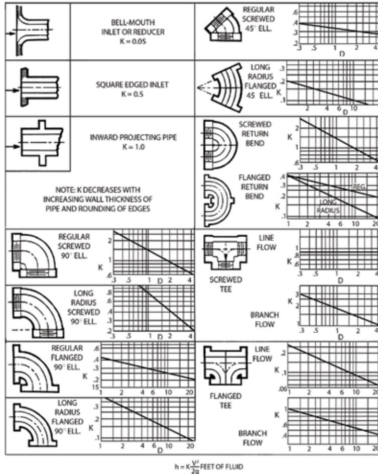
**Figure 6-2 Typical Resistance Coefficients for Valves and Fittings**
