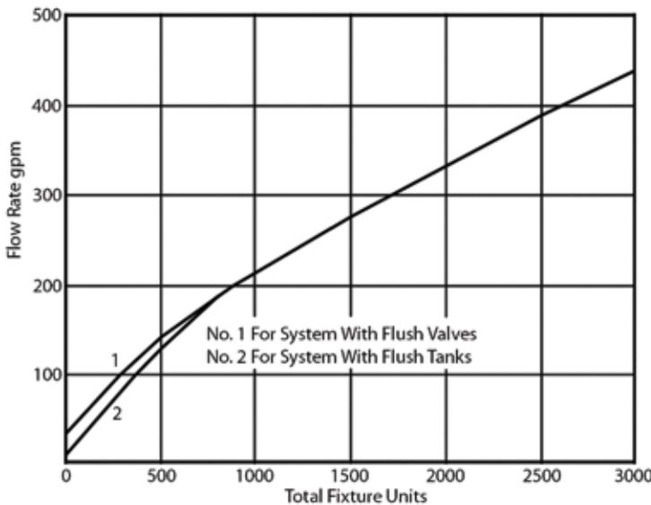
**Figure 6-7 Conversion of Fixture Units to gpm**
