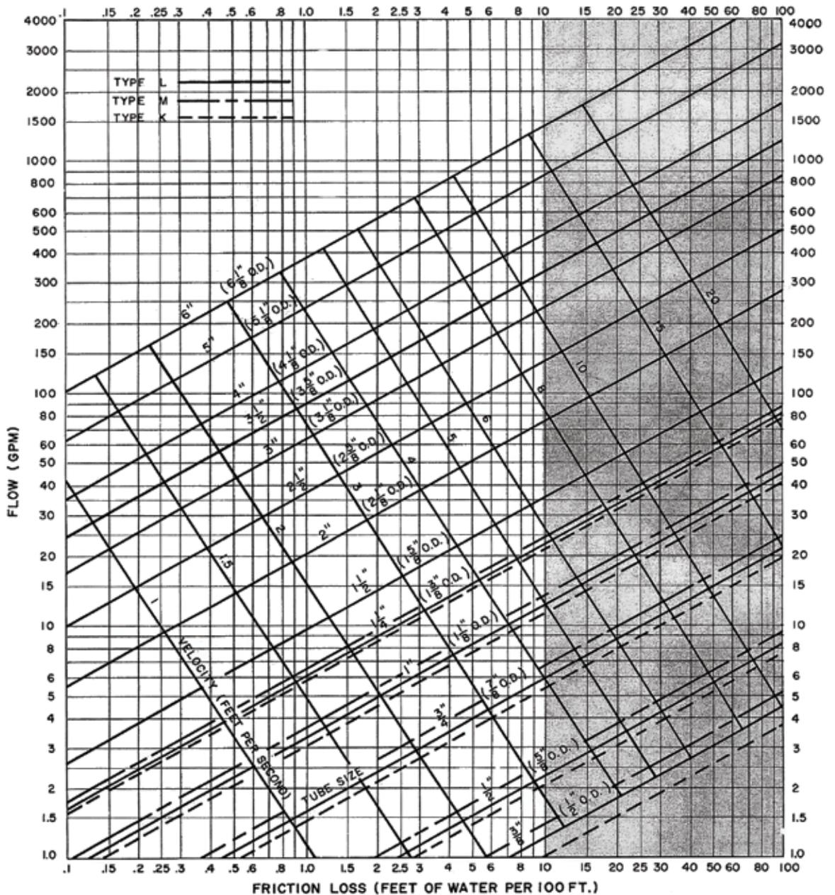
**Figure 6-12 Pipe Sizing Chart for Copper Tubing**
