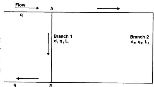
**Figure 6-9 Typical Parallel Pipe Circuit**
