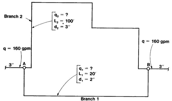
**Figure 6-10 Example of Division of Flow in a Parallel Pipe Circuit**
