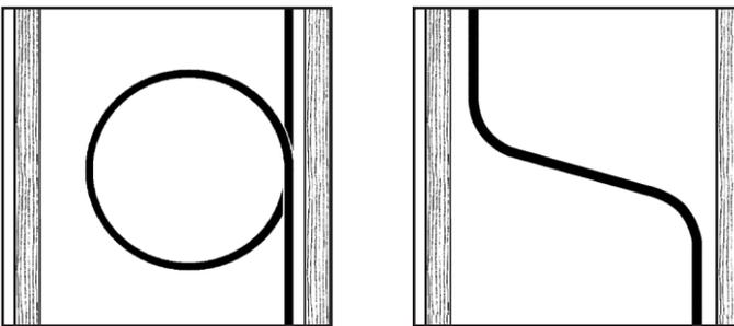
*Expansion loops (left) and offsets (right) also provide means to accommodate tubing expansion and contraction. Refer to the PEX tubing manufacturer's installation instructions for more detailed information on expansion compensation techniques.*
