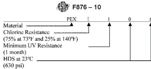
For example ASTM F876 PEX tubing marked with the material designation code PEX 1106 is a PEX tubing meeting the chlorine resistance requirement for 25% of the time at 140°F and 75% of the time at 73°F having a Minimum UV resistance of 1 month and having an HDS for water at 73°F of 630psi (HDB of 1250 psi).
