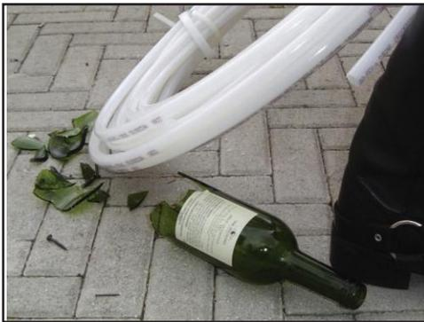
Do not drag the tubing over rough terrain, rocks, or any surface that can cut, puncture, or damage the tubing wall.
