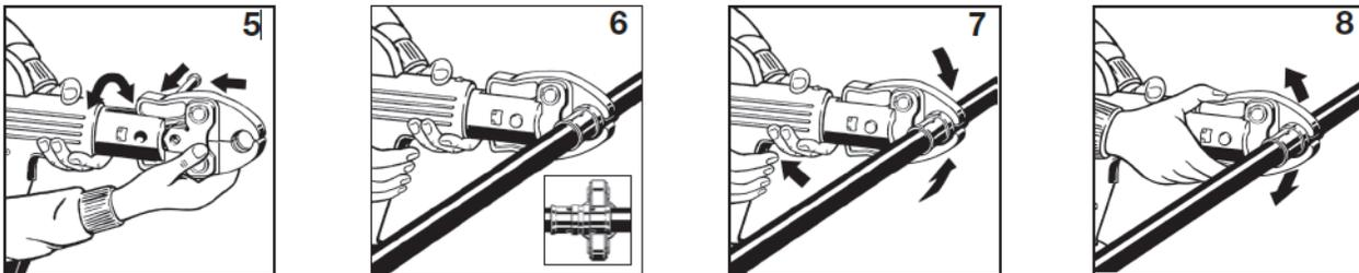
5. Insert the appropriate PEX Press jaw into the press tool and push in the holding pin until it locks.
