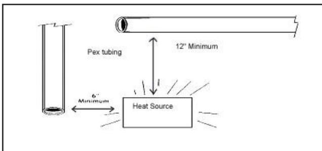
Do not install PEX tubing downstream of any instantaneous, point-of-use or immersed coil water heater where the output is uncontrolled or temperature can exceed 180°F. Contact manufacturer for recommended metallic transition fittings.
