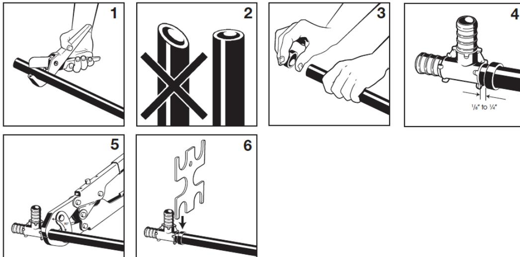
1. The tubing should be cut squarely and evenly without burrs. Uneven, jagged or irregular cuts will produce unsatisfactory connections.
