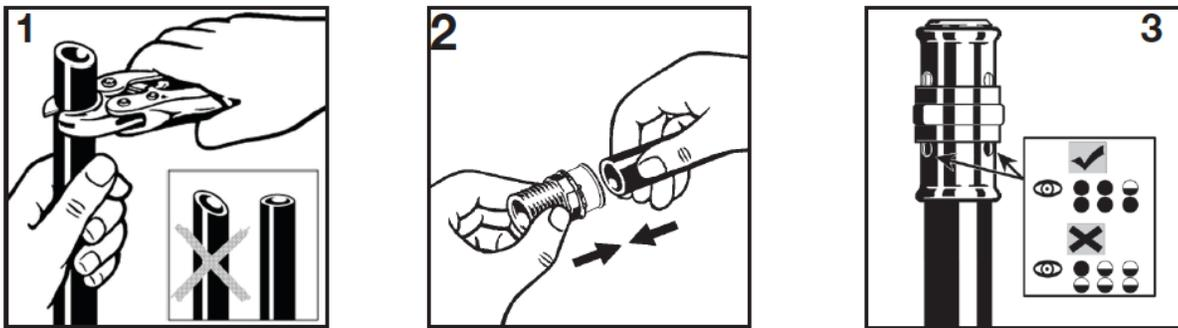
1. Square off tubing to proper length. Uneven, jagged or irregular cuts will produce unsatisfactory connections.
