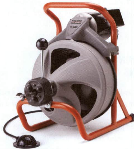
Figure 17-9 Small-diameter cable machines usually have a foot-control device to operate the rotation of the machine (Courtesy of Ridge Tool Company [RIDGID])
