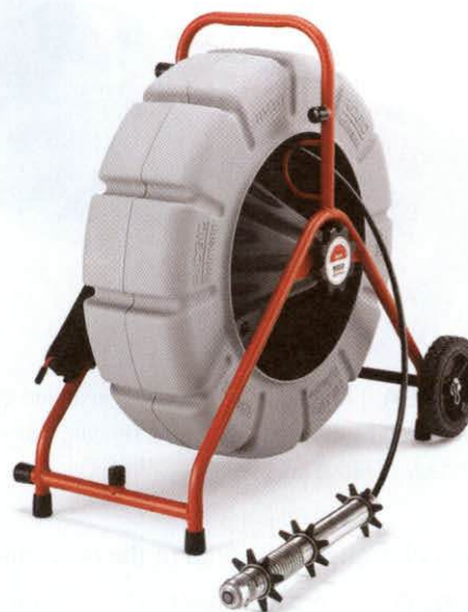
Figure 17-13 A drain or sewer can be inspected with the use of a specialized camera (Courtesy of Ridge Tool Company [RIDGID])
