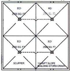
B. Minimum Horizontal Drain Size Roof Area = 2500 sq. ft.
