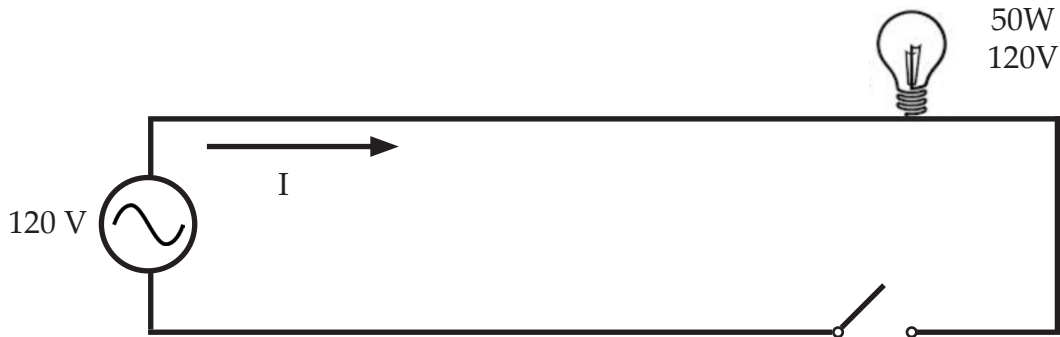
Figure 1A: Simple Circuit - Switch Open The Current (I) is zero I = 0 Amps
