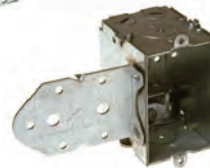
"LB" Bracket Face mounts on front edge of wood stud. Use when space between studs is limited. 5/8" offset to clear narrow door molding.
