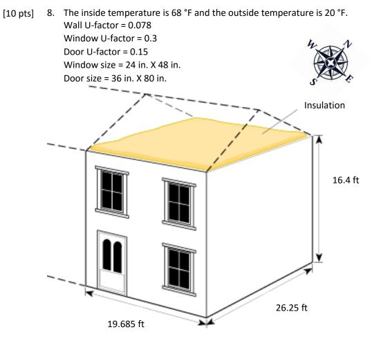
A. Determine the heat loss in the south wall.
