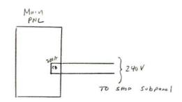
A. What size THHN 75°C CU wire is required for the feeders (conductors) to the subpanel and where in the NEC is the answer found?
