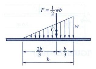
Example 7: Replace the loading on the beam with an equivalent resultant force and specify its location with respect to point A.
