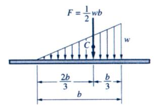
Example 7: Replace the loading on the beam with an equivalent resultant force and specify its location with respect to point A.
