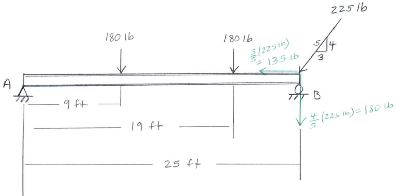
2. Determine the magnitude, direction, and location of the resultant for the non-concurrent force system shown. Locate the resultant with respect to point A. Round all answers to whole numbers.
