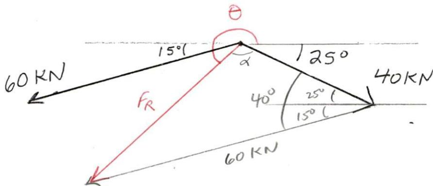
$$F_R = \sqrt{60\text{ kN}^2 + 40\text{ kN}^2 - 2(60\text{ kN})(40\text{ kN}) \cos 40^\circ}$$
