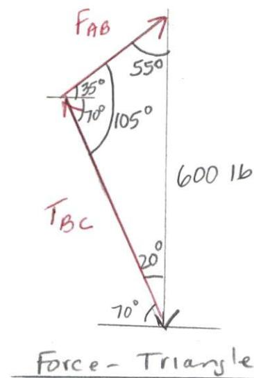
Step 3: Solve for  $F_{AB}$  and  $T_{BC}$  using the force-triangle and trig.
