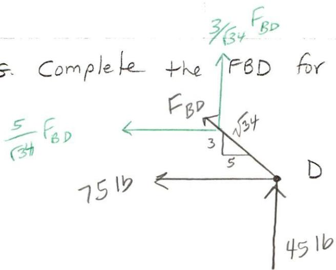
H. Using the FBD for Joint D determine the force in member BD
