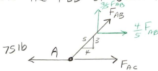
D. Using the FBD for Joint A determine the force in members AB and AC.
