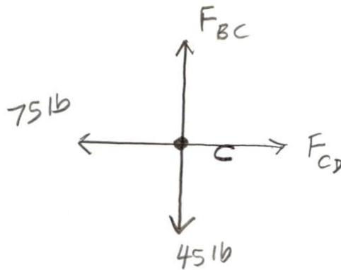
F. using the FBD for Joint C determine the force in members BC and CD.
