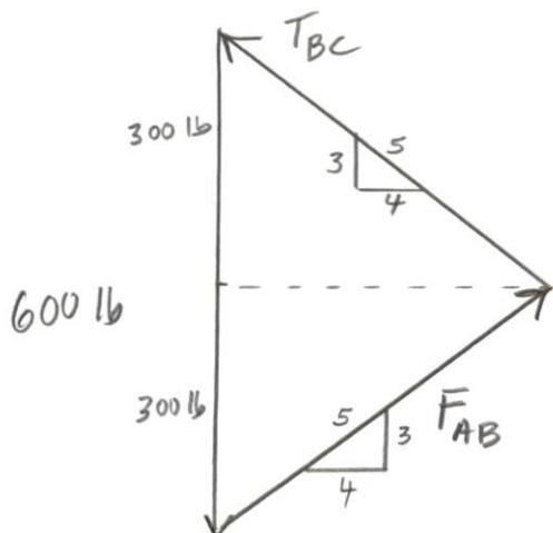
$$\begin{aligned}\delta &= \frac{PL}{AE} \\ &= \frac{500 \text{ lb} \left( 5 \text{ ft} \times \frac{12 \text{ in}}{\text{ft}} \right)}{(0.025 \text{ in.}^2) \left( 30 \times 10^6 \frac{\text{lb}}{\text{in.}^2} \right)} \\ &= 0.040 \text{ in. (elongation)}\end{aligned}$$
