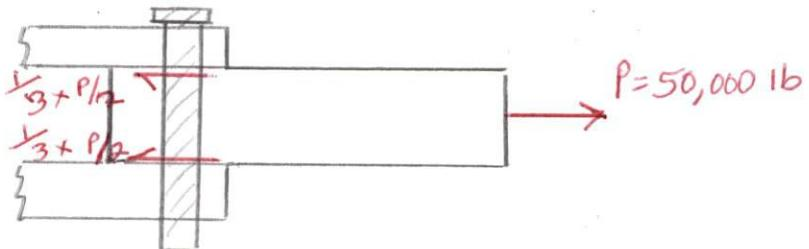
$$\sigma = \frac{P}{A} = \frac{\frac{P}{6}}{\frac{\pi d^2}{4}} = \frac{50,000 \text{ lb}}{\frac{6}{\pi (0.75 \text{ in})^2}} = 18,863 \text{ psi}$$
