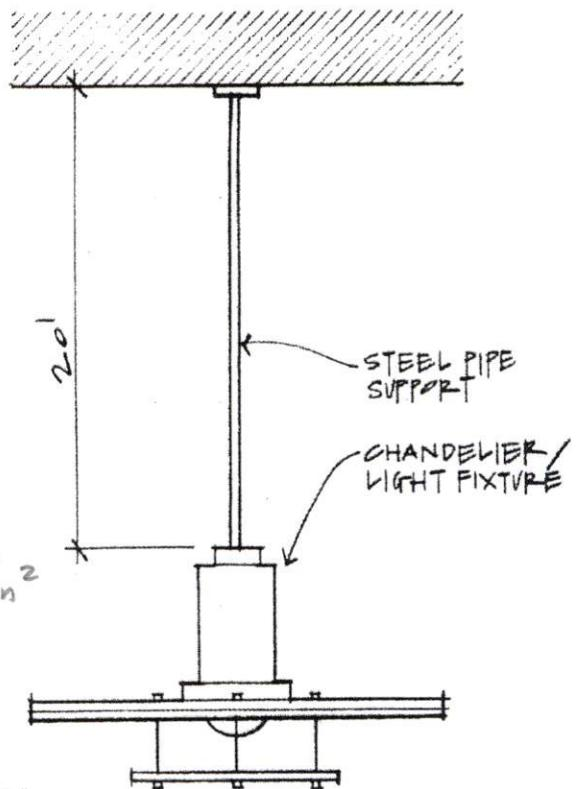
$$(b) \quad \delta = \frac{PL}{AE} = \frac{4500 \text{ lb} (20 \text{ ft}) (12 \text{ in/ft})}{(0.333 \text{ in}^2) \cdot 30,000,000 \text{ lb/in}^2} = \underline{\underline{0.108 \text{ in.}}}$$
