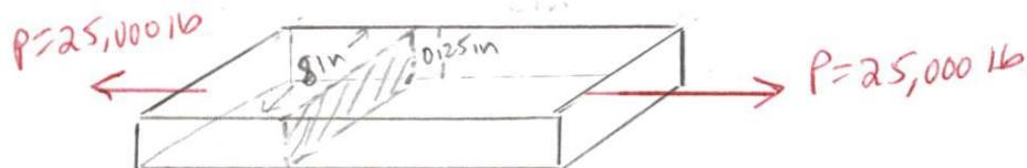
$$\sigma = \frac{P}{A} = \frac{25,000 \text{ lb}}{8 \text{ in} (0.125 \text{ in})} = 12,500 \text{ psi}$$
