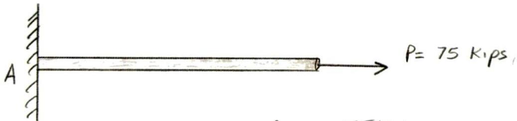
$$\sigma = \frac{P}{A} \Rightarrow A = \frac{P}{\sigma} = \frac{75 \text{ kips}}{35 \text{ ksi/in.}^2} = 2.143 \text{ in.}^2$$
