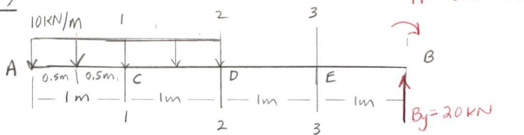
$$V_{1-1} = -\left(\frac{10 \text{ kN}}{\text{m}}\right)(1\text{m}) = -10 \text{ kN}$$
