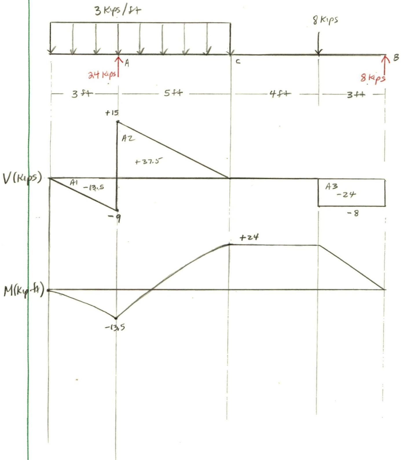
Internal Bending Moment (area under Shear Curve)
