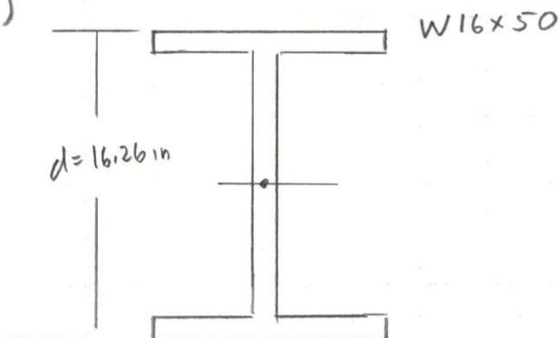
$$\sigma_{MAX} = \frac{M_{MAX}}{S} = \frac{160 \text{ kip} \cdot \text{ft} \left( \frac{12 \text{ in.}}{\text{ft}} \right)}{81 \text{ in.}^3} = 23.7 \text{ ksi}$$
