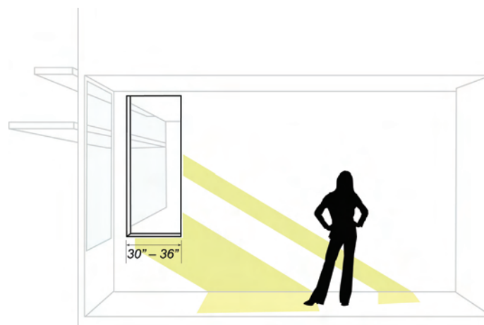
Figure 5-20. (DL11) Transparent partitioning wall.
