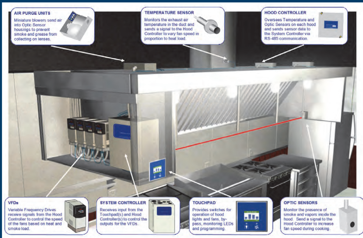
Demand-Controlled Kitchen Ventilation System Overview Image reproduced with permission of Melink Corporation, Intelli-Hood®
