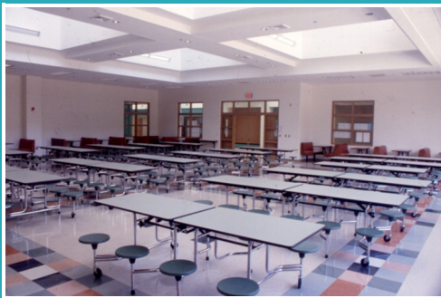
Cafeterias and Multipurpose Rooms with Roof Monitors
