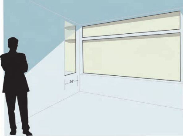
Figure 5-22 (DL10) Maximized Window Width
