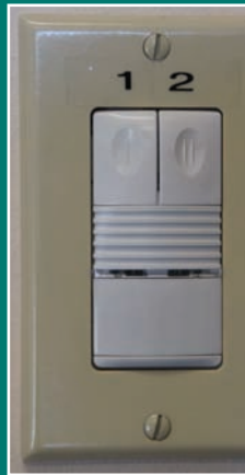
Dual-Circuit Occupancy Sensor Source: Michael Lane, Lighting Design Lab
